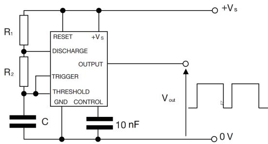
NB IN ASTABLE, TRIG+THRESH are connected to each other.
